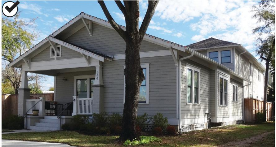
*The walls of this appropriate two-story addition are inset from the historic building, so that the original rear corners remain visible. The side wall addition is small and preserves the original eave line.*
